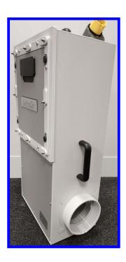
The AstroAir range of air movers has been designed to provide a lightweight yet robust solution for negative pressure within the asbestos removal industry. Manufactured from 5mm AB5 thermoplastic sheets bonded to form triple welds. Switchgear, manometers etc can be removed and replaced without disturbing the integrity of the HEPA filter.
